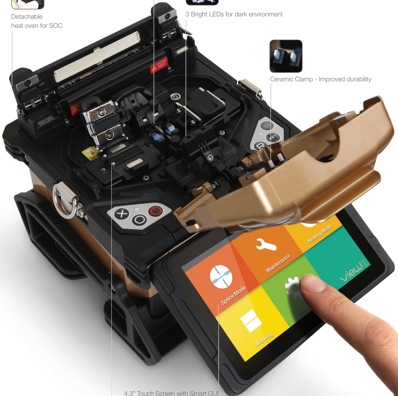
Changeable holder for multi-functional splicing
